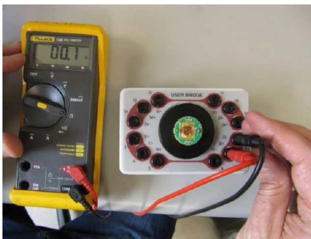
Figure 10. Testing connections using the P150 wiring test station and a hand-held multimeter.
