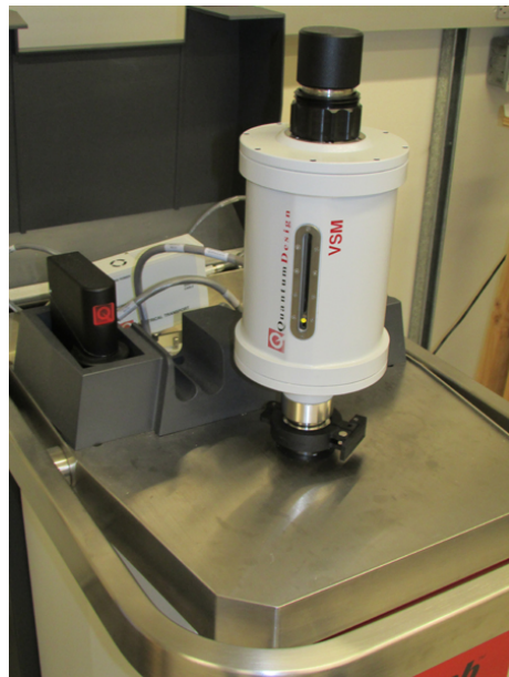
Figure 7: VSM Installed on the VersaLab. Note: the black cap on top can be removed and this is where the sample rod is inserted.
